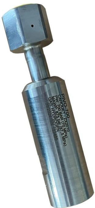
The PIVO-700 swivel fitting connector is designed to protect any device at risk of being subjected to torque during handling. Installed on a fixed component (e.g. a high-pressure collector), its swivel function eliminates any risk of torsion that could damage or shorten the life of the equipment.
